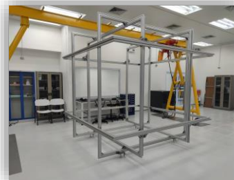
5). Helmholtz Coil for Earth Magnetic field Simulation (Software and Hardware) NARIT-Mechatronics Labs & Research Group
